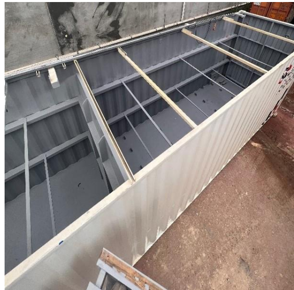
Waste Water Treatment Containers
